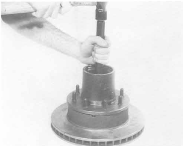
Figure 10 1022-10 Assemble outer wheel bearing cup. Tools: D-254 Installer, C-4171 Handle.
