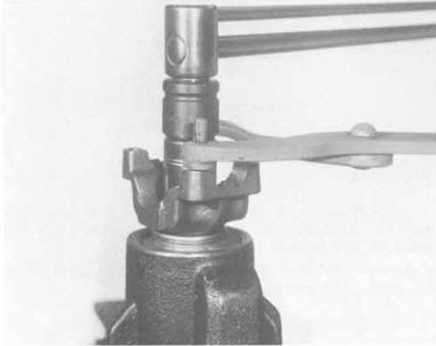
Figure 88 1022-88 Torque pinion nut to 200-220 lbs. ft. (271-298 N•m). Tools: C-4053 Torque Wrench, C-3281 Holder.
