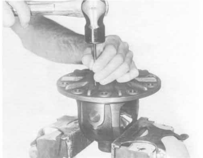
Figure 90 1022-90 Position the differential case in a vise and drive out the lock pin which secures the pinion mate shaft to the case. Use a small drift as shown.
