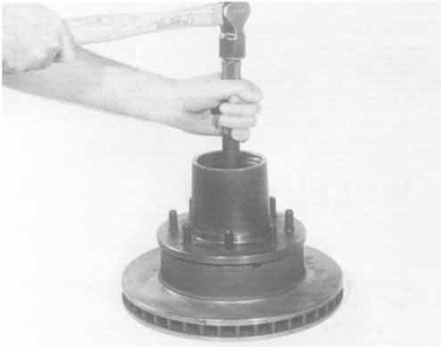
Figure 9 1022-9 Remove inner wheel bearing cup. Tools: D-257 Bearing Cup Remover, C-4171 Handle.
