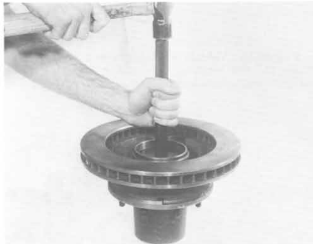
Figure 11 1022-11 Assemble inner wheel bearing cup. Tools: D-256 Installer, C-4171 Handle. Distribute a sufficient amount of grease inside the hub between the bearing cups. Pack inner bearing cone full with the specified grease. Wipe the excess grease around the rollers. Assemble inner wheel bearing cone into cup.
