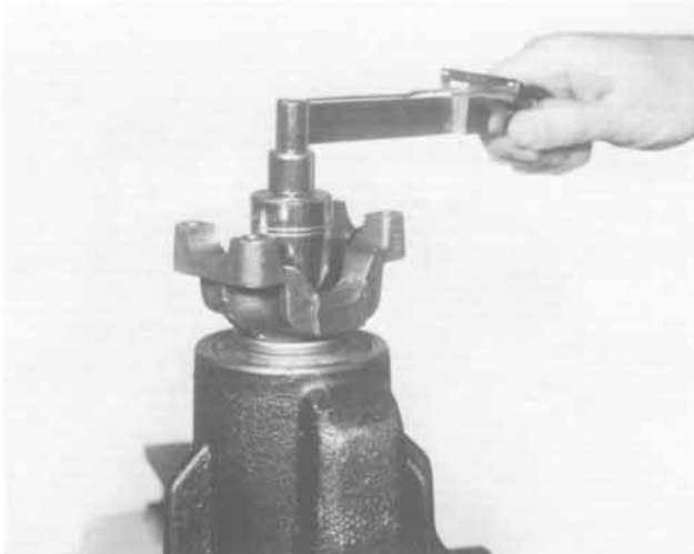
Figure 89 1022-89 Using an inch pound torque wrench as shown, rotating torque of pinion should read 20-40 lbs. in. (2.3-4.5 N•m) with new bearings. To increase preload, remove shims; to decrease preload, add shims. Tool: D-193 Torque Wrench.
